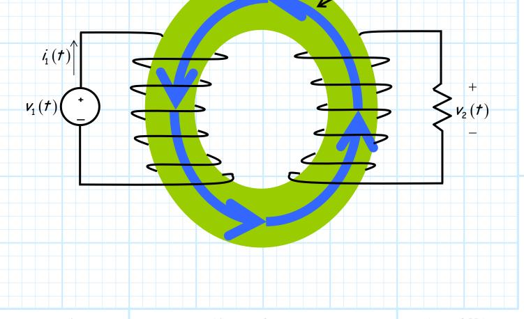
Therefore, we find that the magnetic flux density in the **secondary** solenoid is **equal** to that produced in the **primary**!
